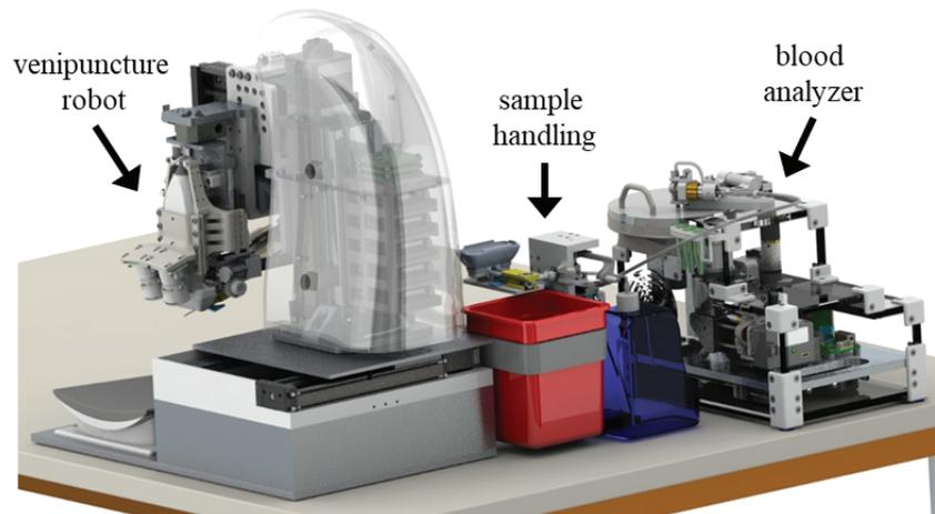
*Design of the automated blood testing and analysis device. The main subsystems include a venipuncture robot, sample handling module, and blood analyzer.*
