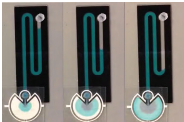
A hydraulic battery pumping fluid through a simple microchannel at a constant rate of 0.6 \mu\text{l}/\text{min} . Each snapshot is 12 min apart (left to right).
