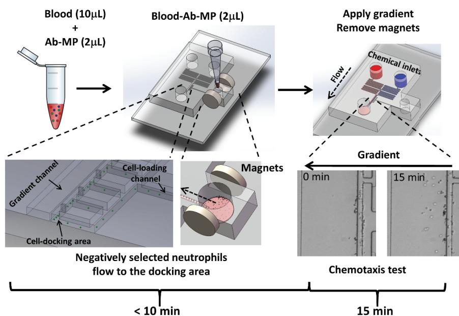
*Illustration of the all-on-chip method for neutrophil chemotaxis analysis using the microfluidic device. Ab-MP: antibody cocktail-magnetic particles.*
