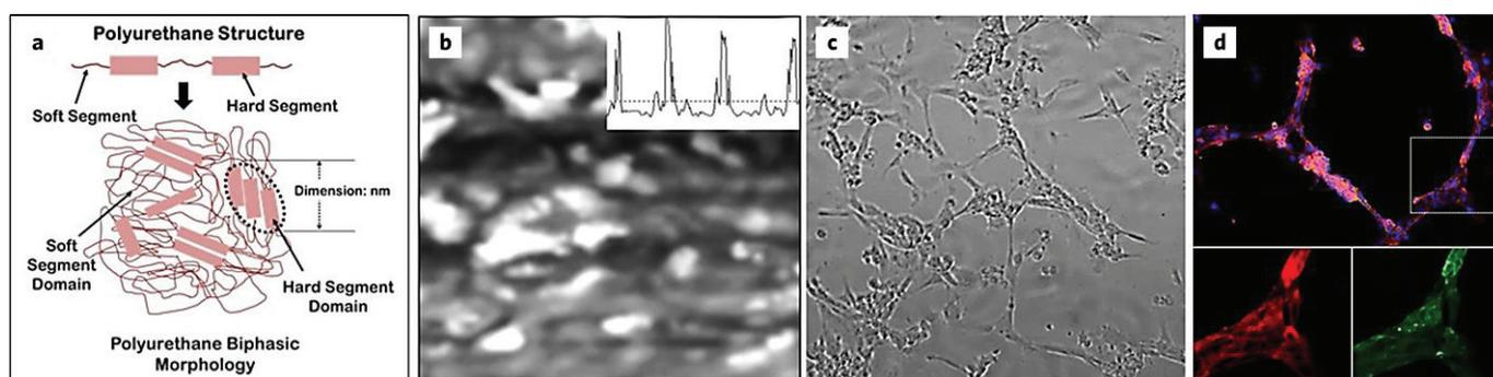
*Polyurethane phase morphology induces endothelial cell organization. a) Segmental composition of polyurethane induces nanostructured phase morphology. b) Atomic force microscopic image of polyurethane phases. c) Endothelial cells organize to form interconnected network like structure on polyurethane matrix. d) Endothelial networks are synchronized by balanced cell-matrix and cell-cell adhesion.*
