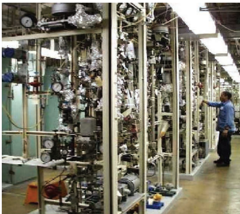
Image 2. Pilot-plant hydrotreating, conducted at Intertek-PARC, Harmarville, Pennsylvania.
