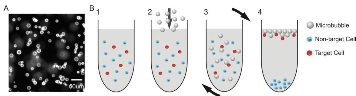
(A) Image of glass microbubbles labeled with PE-conjugated biotin. (B) Schematic of buoyancy activated cell sorting (BACS). Surface-functionalized glass microbubbles bind to target cells after a brief rotary mixing (1–3). Cells attached by glass microbubbles float and are separated spontaneously by buoyancy (4).
