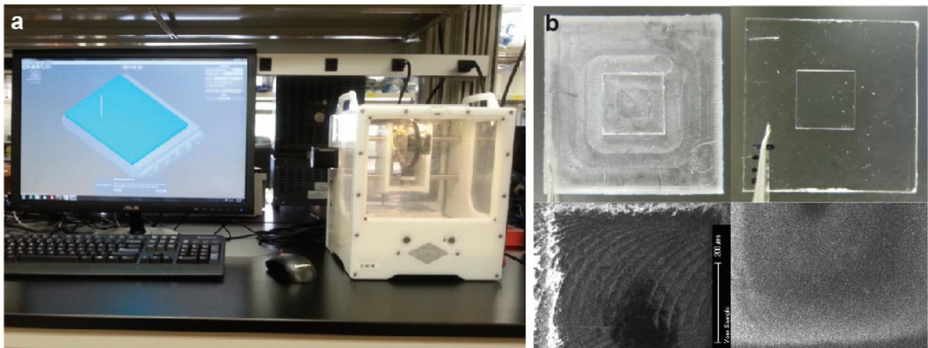
*An economical, user-friendly desktop milling platform for biomedical microdevice fabrication. (a) Othermill V2 and its software interface. (b) Mechanical and chemical polishing improves surface roughness and optical transparency of milled polycarbonate (left: milled surface; right: mechanically and chemically polished; top: gross optical quality; bottom: scanning electron microscopy of the surface)*
