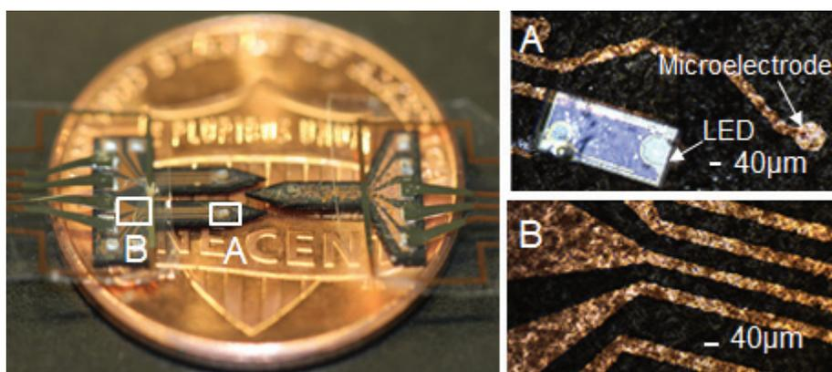
*Microfabricated single- and dual-shank polycrystalline diamond based optrodes: A. Integrated microscale light-emitting diode and recording microelectrode. B. Metal pads and interconnect wires.*
