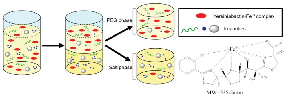
*A diagram of the aqueous two phase system (composed of poly(ethylene glycol) [PEG] and salt phases) used to pre-purify yersiniabactin from the crude extract of a cellular culture used to produce the compound. The compound, complexed to iron, is separated and concentrated into the PEG phase of the system and simplifies and improves subsequent steps at final purification.*
