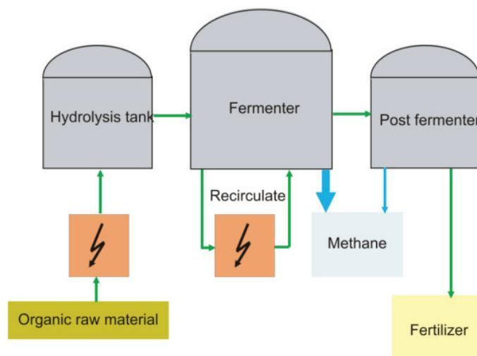
*Possible arrangement of electric treatment within the biogas process: High pulse energies are for raw substrate treatment yielding a high level of cell killing and disintegration while moderate pulse protocols are used for recirculate where the focus lies on the control of the microbial community.*
