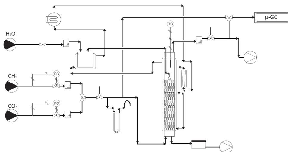
*Flowsheet of the experimental apparatus used for the absorption study and main results obtained in term of difference between the carbon dioxide concentration entering and exiting from the column depending on the different experimental conditions.*
